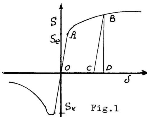
Segment O-C indicates the plastic deformation  $\bar{\delta}$ , at B, which at the time the load is relieved remains unaltered; segment C-D represents the elastic deformation  $\delta_e$ . If the bar is isolated for  $S=0$ ,  $\delta=\bar{\delta}$ ; if it is within a hyperstatic system, for  $S=0$ ,  $\delta=\bar{\delta}+\bar{\delta}_e$ , where  $\bar{\delta}_e$  indicates the elastic deformation constrained within the system and recoverably only through cutting the bar.
