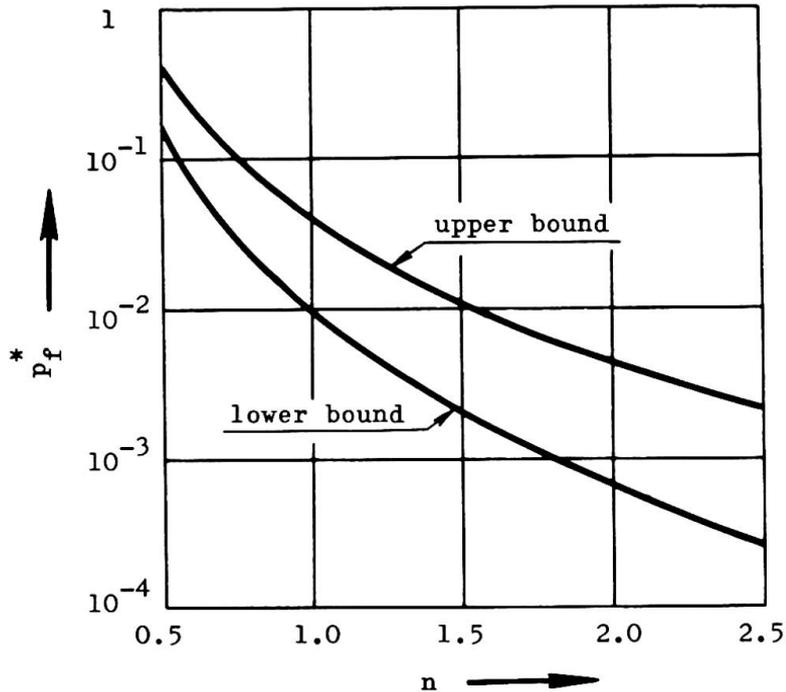
Fig. 1 Probability of Failure  $p_f^*$  as a function of safety factor  $n$
