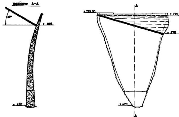
Fig. 13 Vajont Dam. Asymmetric slide material acting on upstream face.
