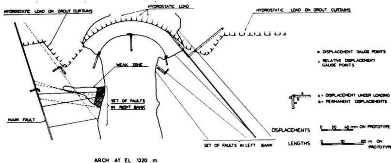
Fig.5 Kurobe IV Dam. Displacements recorded at a horizontal section (el. 1320 m).
