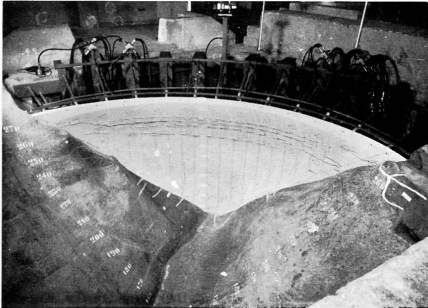
Fig. 8 Flumendosa Dam. Downstream view of model under test.
