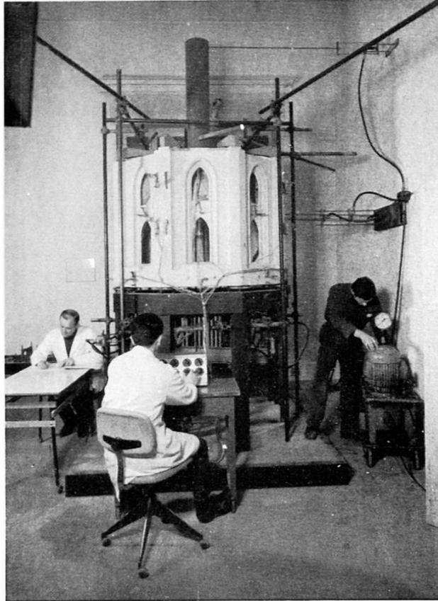
Fig. 11 Milan Cathedral. Elastic model of masonry dome.
