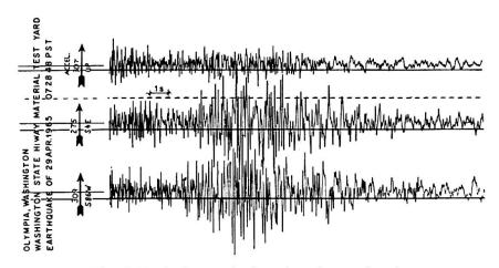
Fig. 6. Typical record of earthquake acceleration
