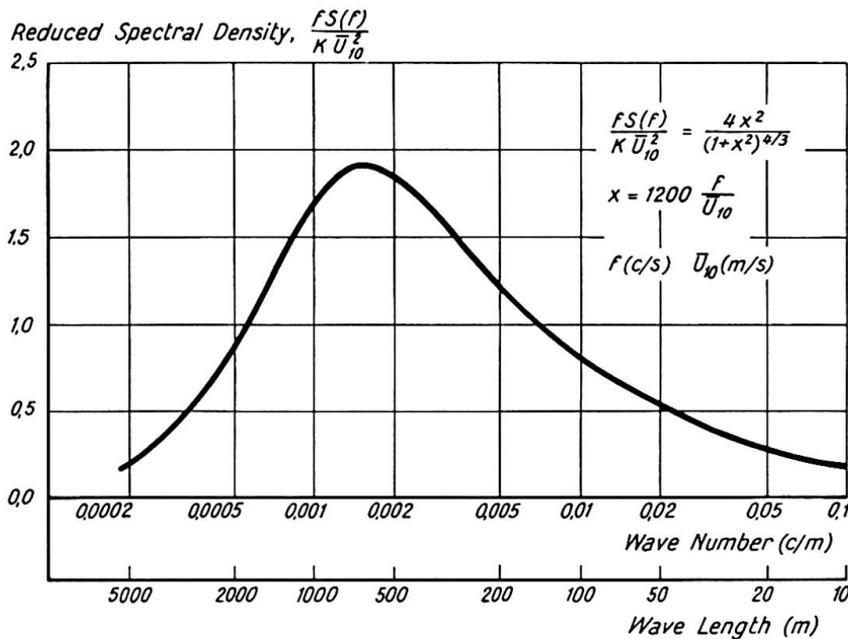
Fig. 3. Spectral density of longitudinal component of wind velocity according do Davenport [8]
