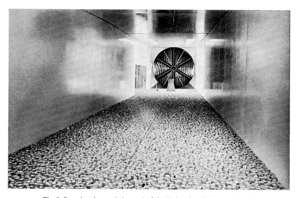
Fig. 5. Boundary-layer wind tunnel of the University of Western Ontario
