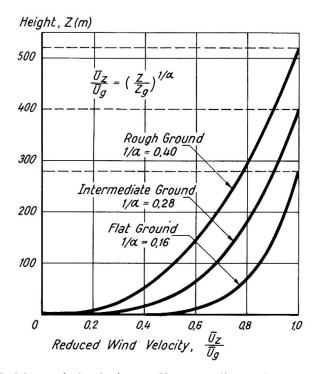
Fig. 2. Mean wind velocity profiles according to Davenport [8]
