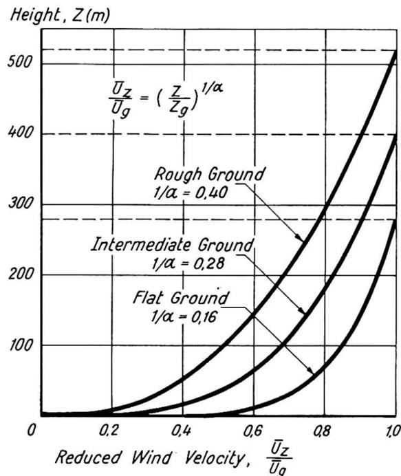
Fig. 2. Mean wind velocity profiles according to Davenport [8]
