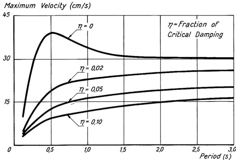
Fig. 7. Spectra of maximum velocities according to Housner [27]
