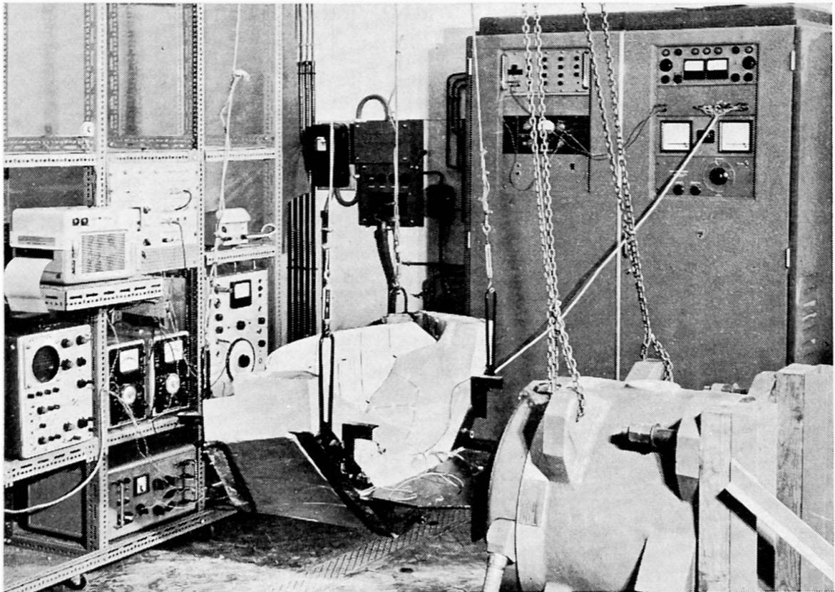
Fig. 10. Random-vibration set-up for model testing
