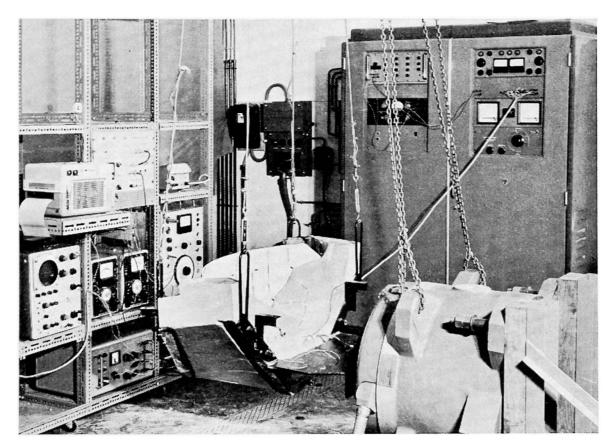
Fig. 10. Random-vibration set-up for model testing
