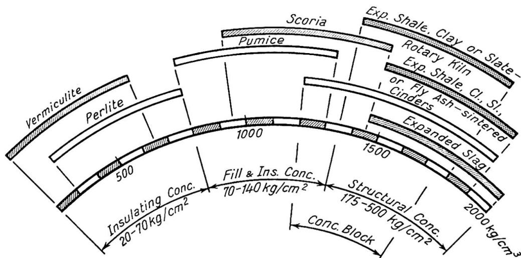
Fig. 1. Spectrum of Lightweight Aggregate Concretes
