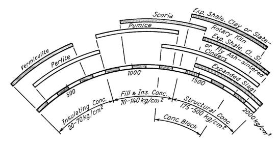
Fig. 1. Spectrum of Lightweight Aggregate Concretes
