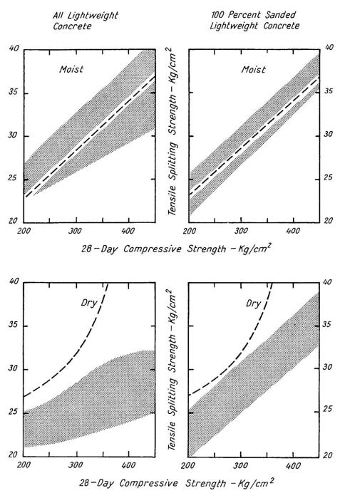
Fig. 4. Tensile Splitting Strength
