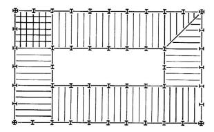
Fig. 2. Typical Plan Showing Various Possible Corner Framings
