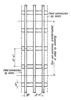
Fig. 8. Prefabricated Units for Framed Tube Type Structures
