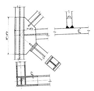
Fig. 9. Schematic Joint Detail for Optimum Truss Type Structures
