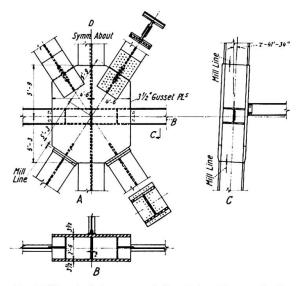
Fig. 10. Difficult Joint Detail for John Hancock Center
