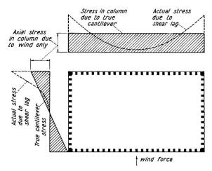
Fig. 4. Shear Lag in Framed Tube
