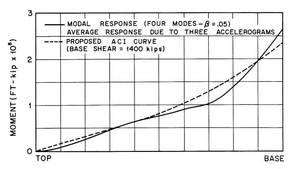
Figure 5 Comparison of Moment Curves - Chimney #4
