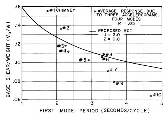
Figure 1 Base Shear/Weight Vs. First Mode Period
