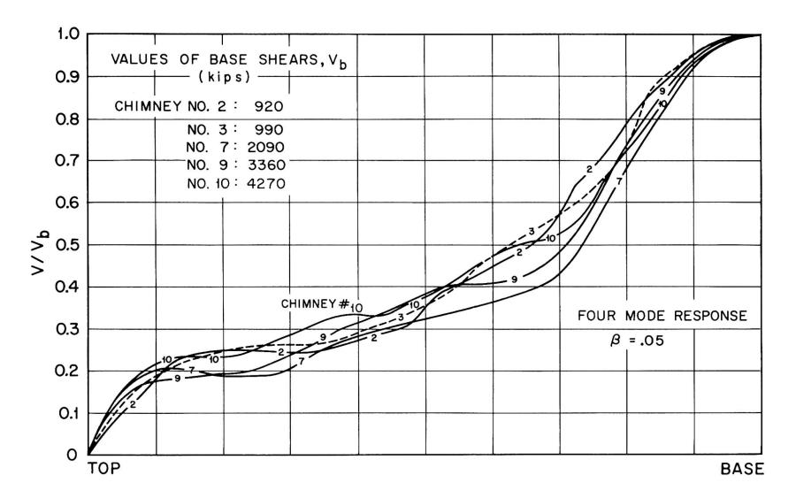
Figure 3 Normalized Maximum Shear Curves (Average Response Due to Three Earthquakes)
