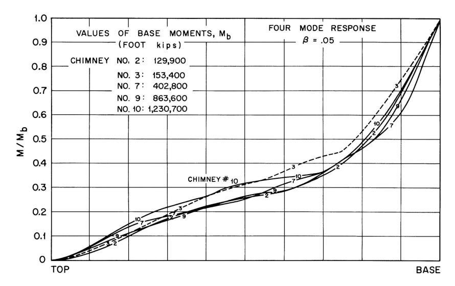
Figure 4 Normalized Maximum Moment Curves (Average Response to Three Earthquakes)
