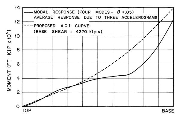
Figure 7 Comparison of Moment Curves-Chimney#10 (Actual Response Vs. Proposed ACI)
