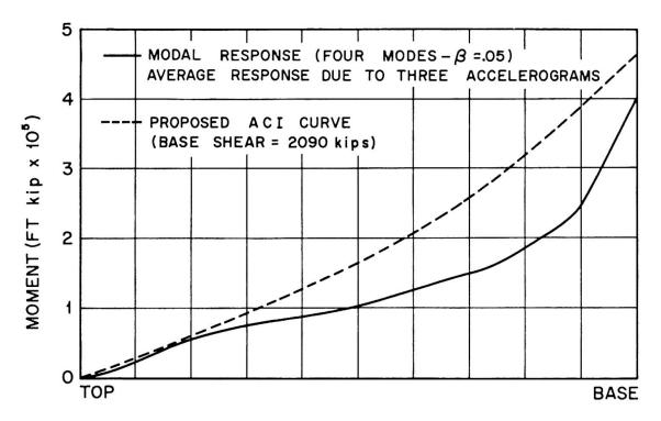
Figure 6 Comparison of Moment Curves-Chimney #7
