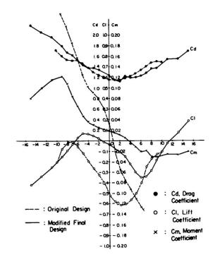
Figure -2 Aerodynamic Coefficients of Girder Section
