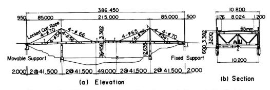
Figure-1 Elevation and Section of Onomichi Bridge
