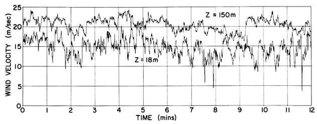
FIG. 6 WIND VELOCITY RECORD FROM I8m AND I50m KSC MET. TOWER
