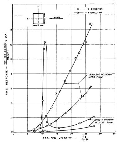
Fig. 4. Response of a Square Cantilevered strongest vibration at Prism in Turbulent and Smooth Flow.
