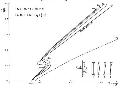
Fig. 2. Universal Galloping Response of Square Cylinders Having Different Normal Modes
