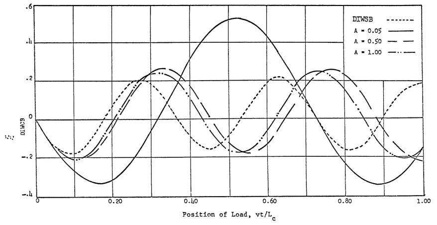
FIG. 3. EFFECT OF RIGIDITY RATIO ON DYNAMIC INCREMENT FOR DEFLECTION AT MIDSPAN CONSTANT MOVING FORCE,  $L_c = r = 200^{\circ}$ ,  $\alpha_v = 0.18$
