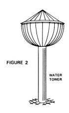
twentieth scale wind tunnel tests were commissioned at the National Physical Laboratory (Smith 1964) and indicated that vortex excited instability was unlikely. Unfortunately it is not yet possible to simulate gusting conditions in a wind tunnel and recourse to calculation was necessary in this respect.
