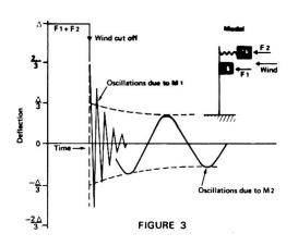
continued for some time afterwards. By monitoring the motion of the tank by sensing the displacement of the stalk and extrapolating the behaviour of the water back to zero time, it was possible to show (Figure 3) that the wind load was distributed approximately two-thirds on to the stalk and one-third on to the flexible tank and water. It is this third of the force which is potentially magnified by the dynamic response of the water and the tank.
