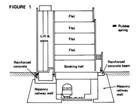
to isolate it from the vibrations generated by the railway. This is probably the first complete building to be isolated in this way from low frequency ground-borne vibrations (Waller 1966).
