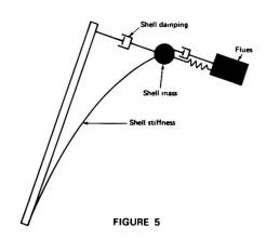
correspond with the flue sections and here again rotational inertia has been allowed for. Hysteretic damping has been included both in the bearings and in the shell. The complete system therefore has been represented by twenty-two masses with associated spring and damping systems.
