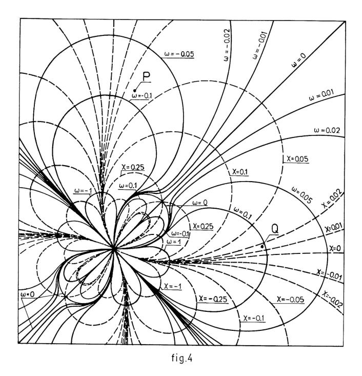
In fig. 4 the curves of constant damping  $\chi$  and their orthogonal trajectories of constant pulsation ware traced in the particular case  $\gamma=\lambda=1, \varepsilon=\pi/2$
