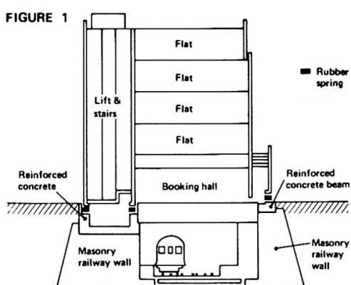
Clearly the introduction of springs for this purpose significantly alters the natural frequencies of the building. In this case the vertical frequency of the system was designed to be 7 Hz. It is a characteristic of the laminated rubber spring that its horizontal stiffness is two orders less than its vertical stiffness so that in the first instance the
