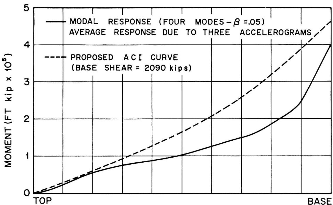
Figure 6 Comparison of Moment Curves - Chimney #7
