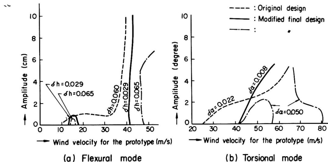
Figure-3 Amplitude and Wind Velocity of Model Vibration
