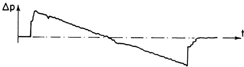
Fig. 1. Pressure signature due to the sonic boom
