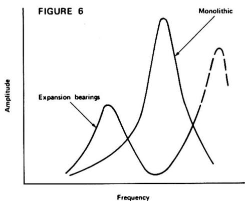
It can be seen that the behaviour of the two systems is entirely different. It was a relatively simple step from knowing the response characteristics of the chimney to calculate its behaviour under gust conditions. This was done by integrating the response spectrum obtained using these frequency characteristics, and the net result showed that the chimney with flexible expansion bearings had in fact a dynamic response of only about half that of the monolithic chimney.
