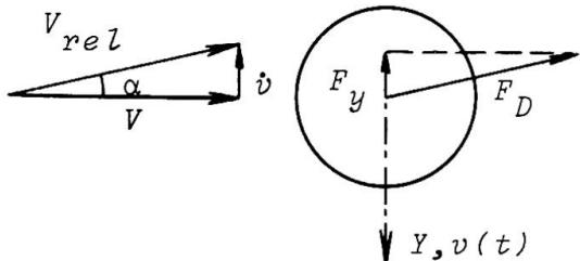
Fig. 6. Vibrating Cylinder in the Flow
