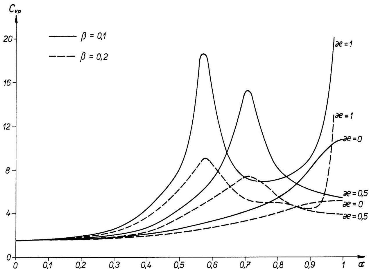
Fig.2. The coefficient  $C_{VP}$  as a function of the velocity parameter  $\alpha$ , damping parameter  $\beta$  and mass parameter  $\alpha_e$
