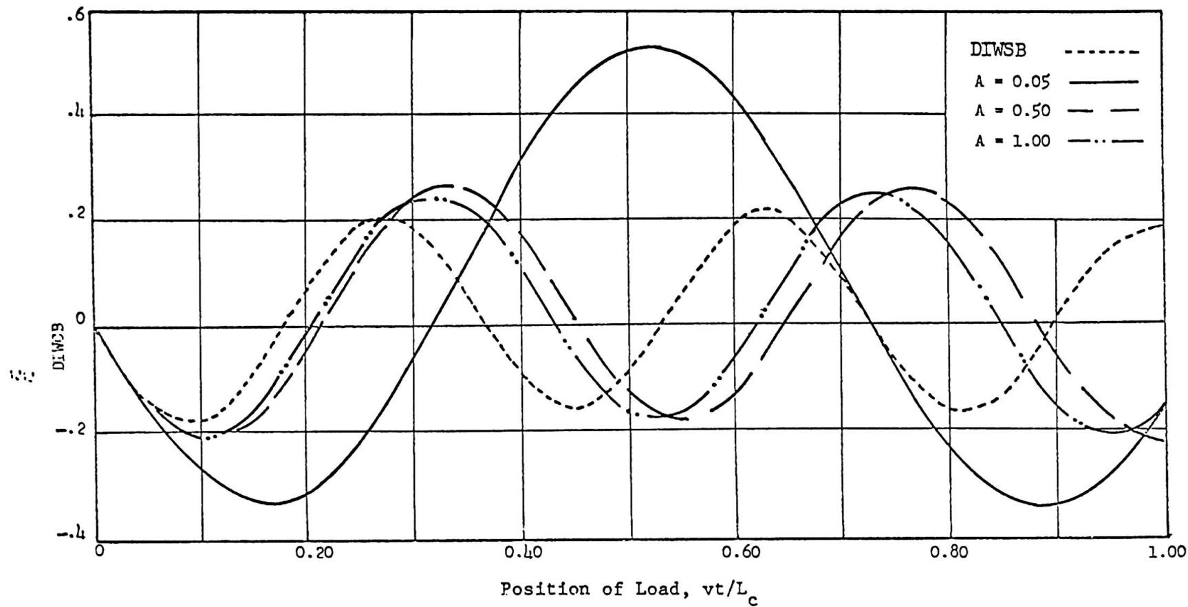
FIG. 3. EFFECT OF RIGIDITY RATIO ON DYNAMIC INCREMENT FOR DEFLECTION AT MIDSPAN
