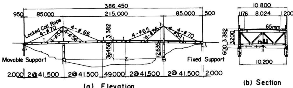
Figure-1 Elevation and Section of Onomichi Bridge
