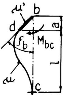
and the rigidity of the pier increases in this part substantially. It can be assumed that the moment of inertia is infinitely large there. The low end was assumed to be fixed rigidly, which holds only when the foundation reposes on solid rock. The end moment acting on the upper end can be expressed by frequency functions  $F(\lambda)$  which have been developed by the author<sup>4)5)</sup>. It is
