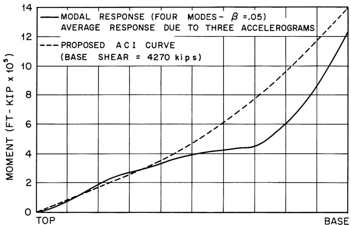
Figure 7 Comparison of Moment Curves-Chimney #10
