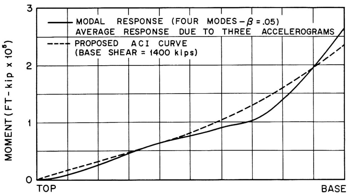
Figure 5 Comparison of Moment Curves - Chimney #4
