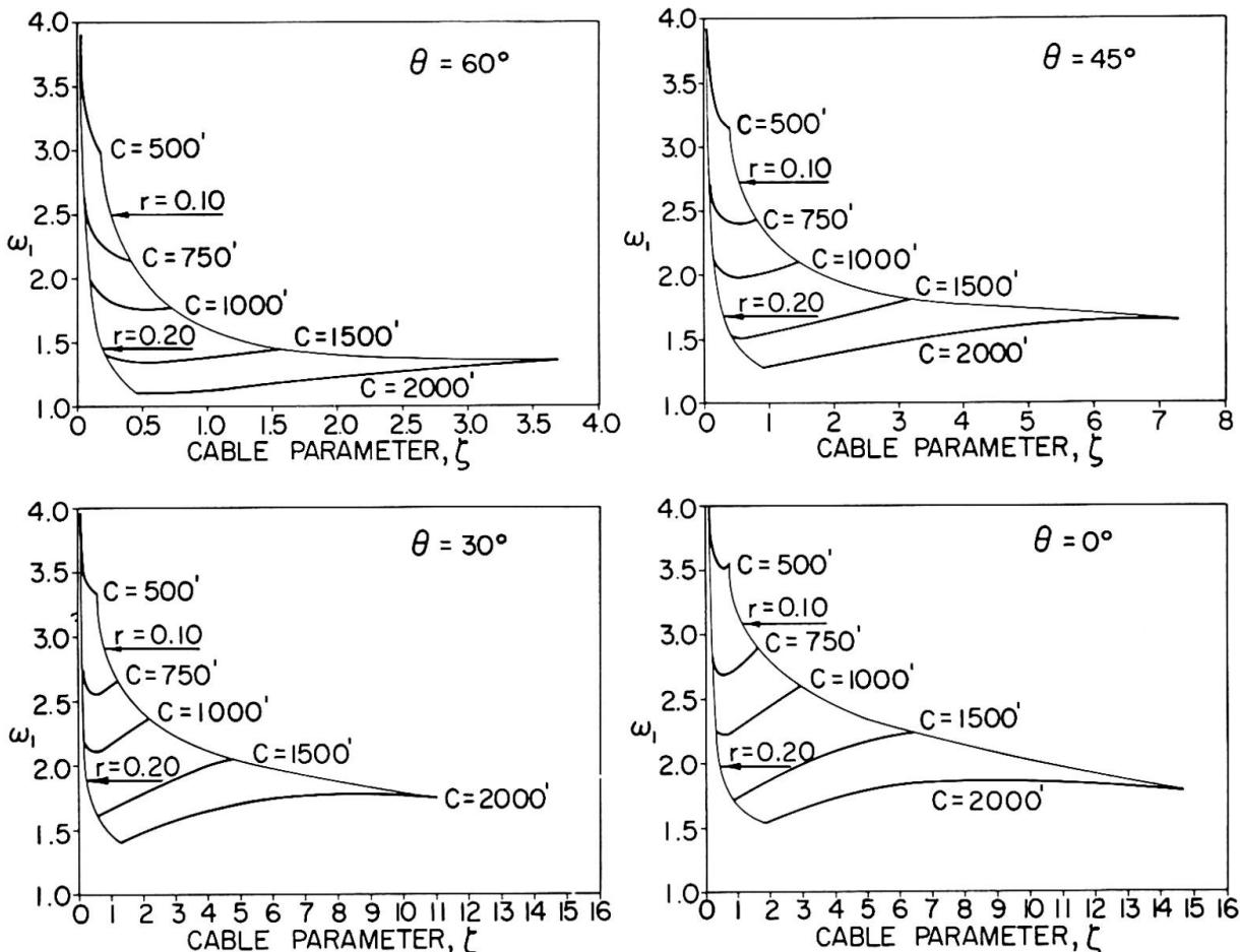
FIG. 4 FIRST NATURAL FREQUENCY  $\omega_1$  (rad/sec) OF GUY CABLES INCLINED AT  $\theta^\circ$ , CROSS-COUPING BETWEEN MODES INCLUDED
