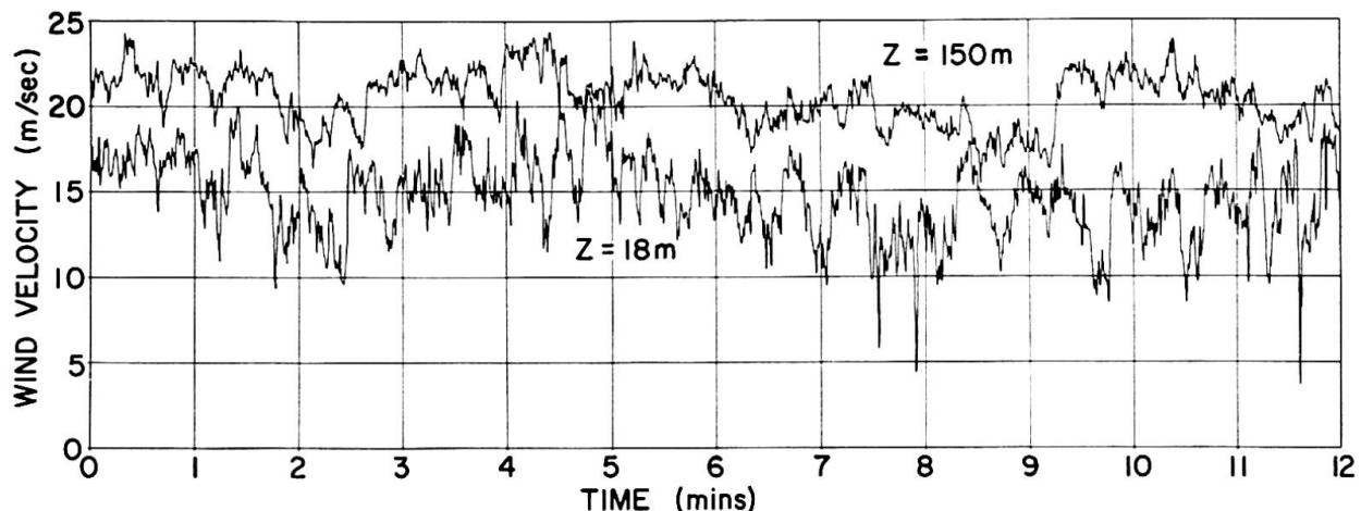
FIG. 6 WIND VELOCITY RECORD FROM 18m AND 150m KSC MET. TOWER
