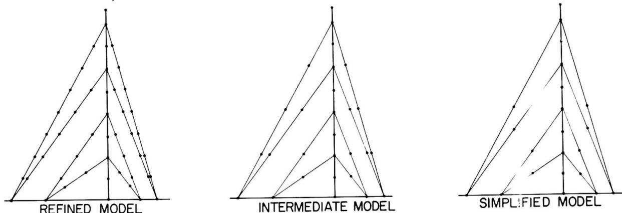
FIG. 7 NODAL POINT ARRANGEMENTS FOR GUYED MAST MODELS
