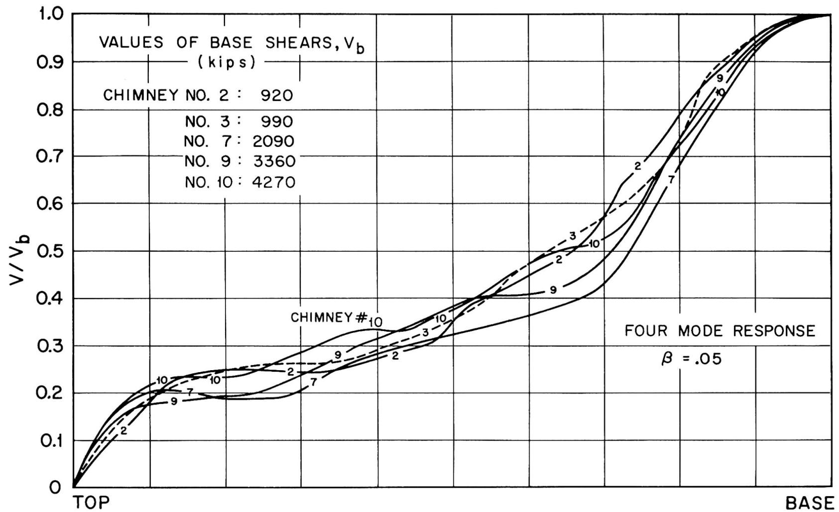
Figure 3 Normalized Maximum Shear Curves
