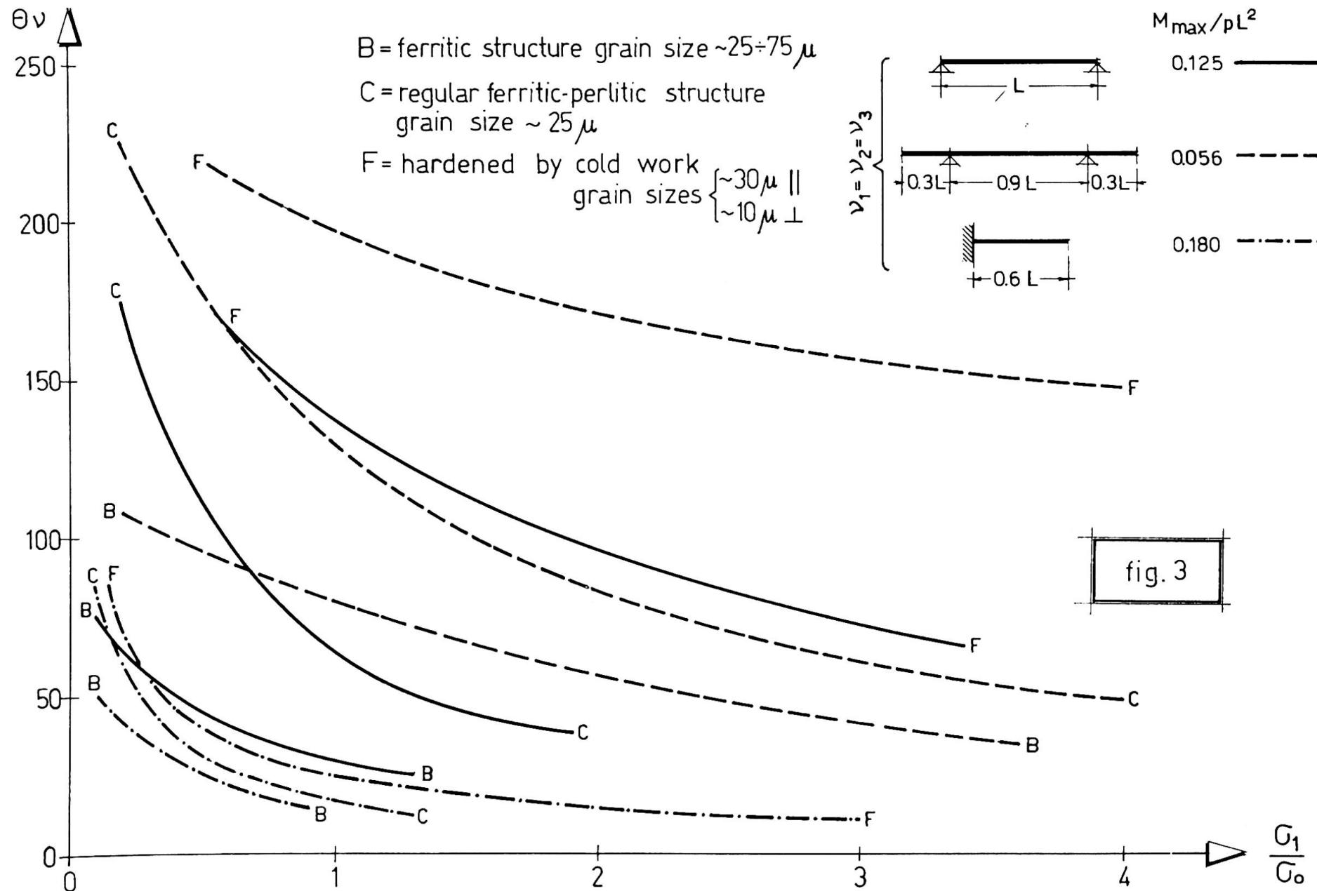
The results appear in fig. 3 where two dimensionless parameters have been introduced:  $\theta \nu$  (a number of cycles) and
