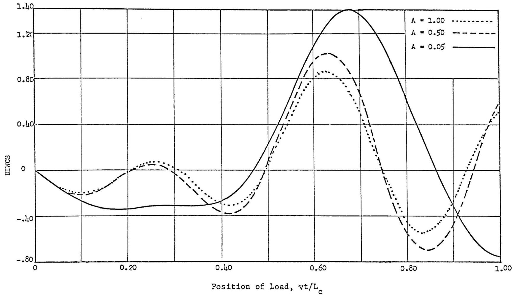
FIG. 4. EFFECT OF RIGIDITY RATIO ON DYNAMIC INCREMENT FOR DEFLECTION AT MIDSPAN
