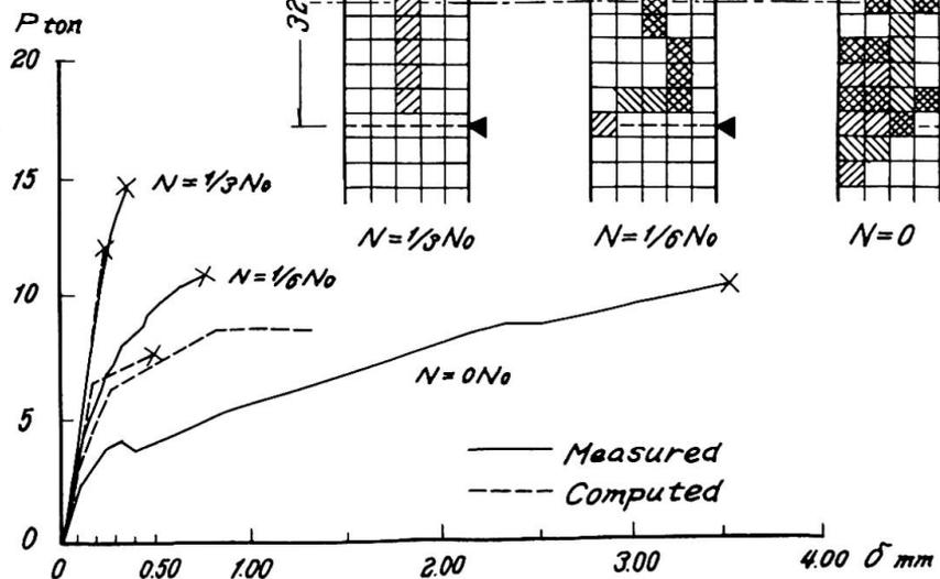
Fig. 10 shows the test results with solid lines and corresponding calculated values of foregoing deformation analysis for the case of a shear span ratio  $a/d=1,2$  and axial load level ratios of 0,  $1/6$  and  $1/3$  with dotted lines.
