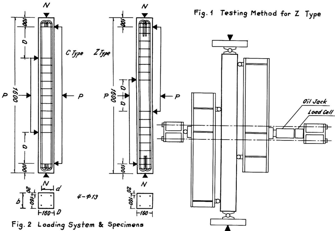
Fig. 2 Loading System &amp; Specimens
