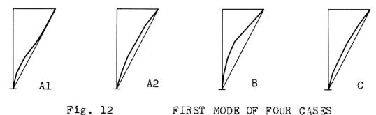
The modes of vibration obtained for the Frames  $A_1$ ,  $A_2$ , B and C are shown in Fig. 12, and the response values in terms of shear force coefficient are shown in Fig. 13.
