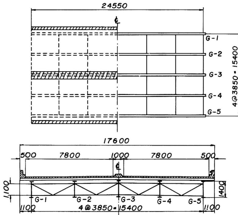
Fig. 5. General view of test bridges
