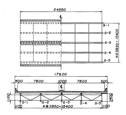
Fig. 5. General view of test bridges
