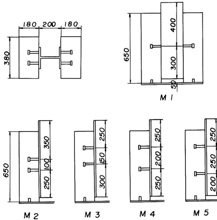
Fig. 1. Push-out specimens
