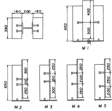
Fig. 1. Push-out specimens
