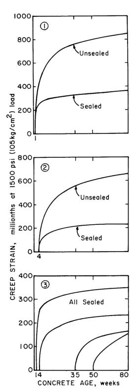
Figs. I, 2, 3 - Creep of Plain Concrete— Effect of Age of Concrete at Loading and Drying Shrinkage.
