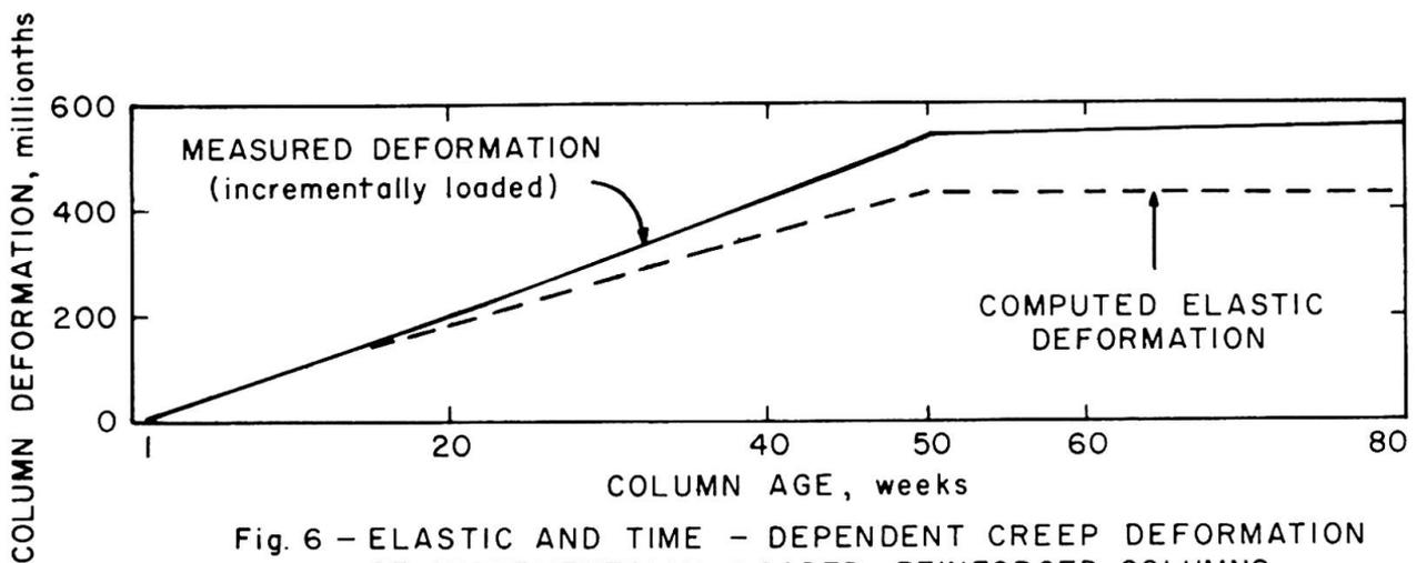
Fig. 6 – ELASTIC AND TIME – DEPENDENT CREEP DEFORMATION OF INCREMENTALLY LOADED REINFORCED COLUMNS
