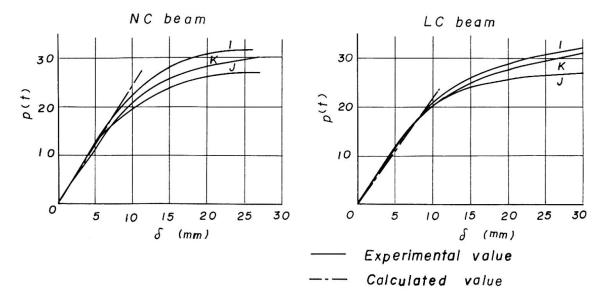
Fig. 3. Deflection of beamsat center
