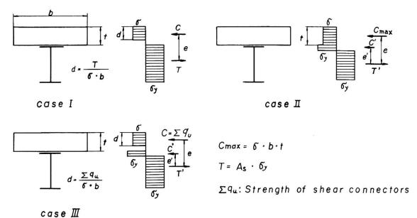
Fig. 4. Calculation method of breaking moment
