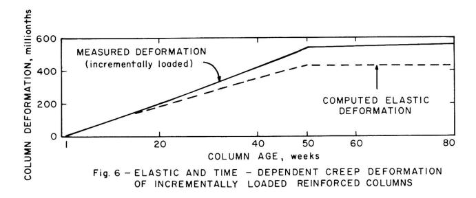
that the influence of creep is small when sealed reinforced columns are incrementally loaded during a long-time period. At an age of 50 weeks the ratio of measured creep strain to computed cumulative elastic strain was 0.25.
