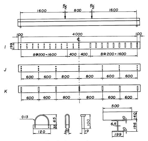
Fig. 2. Beam specimens
