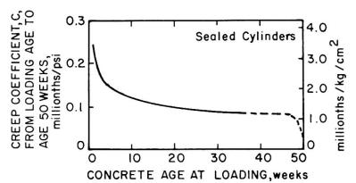
Fig.4-MEASURED CREEP COEFFICIENT
