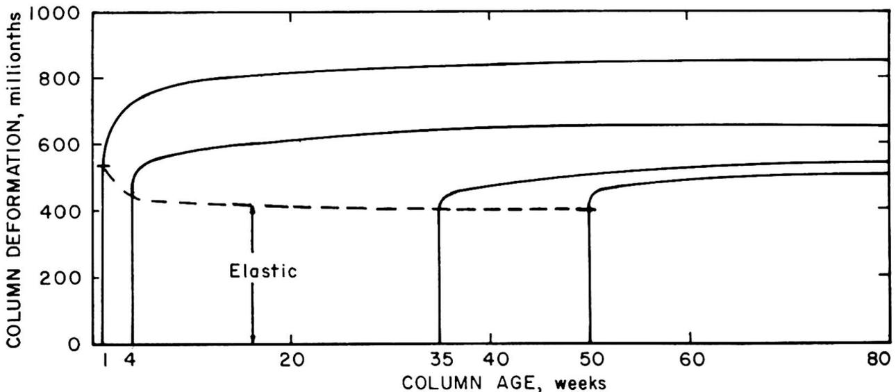
Fig. 5 — ELASTIC AND TIME - DEPENDENT CREEP DEFORMATION OF INSTANTANEOUSLY LOADED REINFORCED COLUMNS
