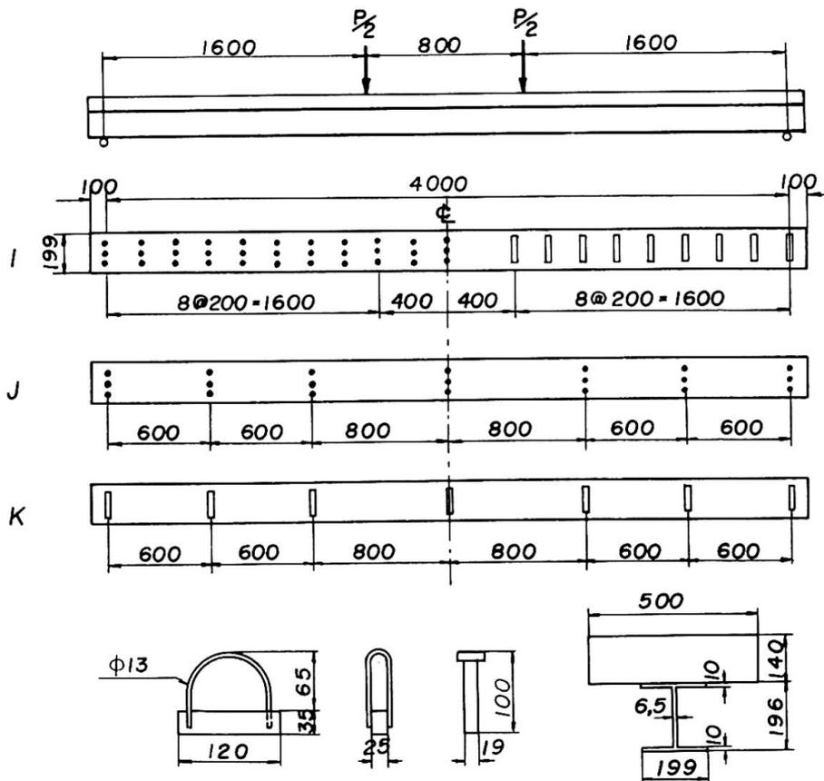
Fig. 2. Beam specimens
