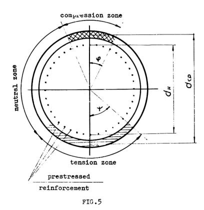
The size of the tensile zone is selected in such a way that it must satisfy the following conditions:  $S_{\delta} = 0.8 S_{0}$ , where S& - the statical moment of compressed zone calculated in relation to the centre of gravity of tensile zone, S - the statical moment of the entire area of concrete situated above the centre of gravity of the tensile zone, related to this centre.
