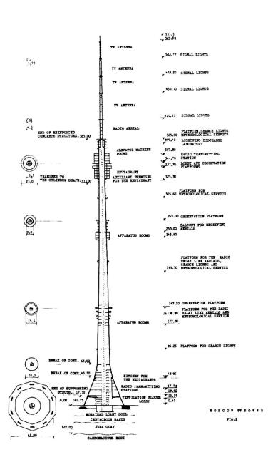
The foundation of the tower has the form of 10-sided polygonal ring slab with an average diametre - 60 m, width 9.5m and the thickness 3 - 5.5 m.
