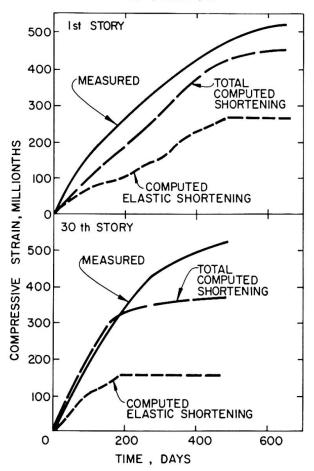
Fig. 5 - Deformation of Columns
