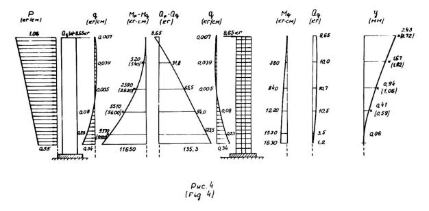
The results of the design of the model under the supposition of embedment of the framework in the plane of the floor over the second floor by formulae (4), the diagrams of loads acting on framing and core, of bending moments and shear forces are given in Fig. 4. On the diagram of bending moments small crosses show the data obtained from the experiment by gauges attached to the core of the building and processed appropriately.
