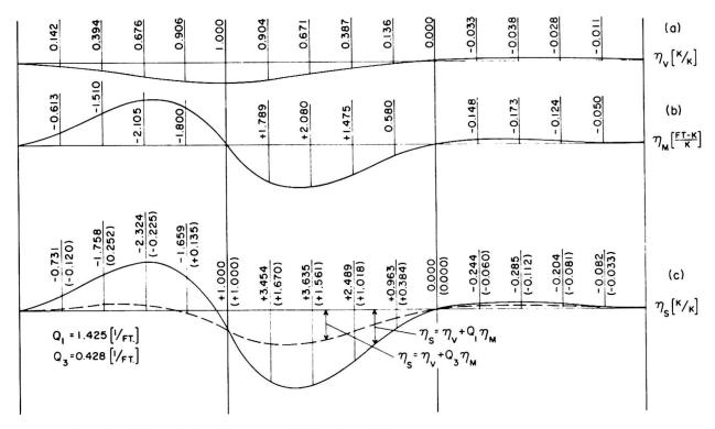
FIG. 4 INFLUENCE LINES FOR MAXIMUM SLAB SHEAR AT COLUMNS
