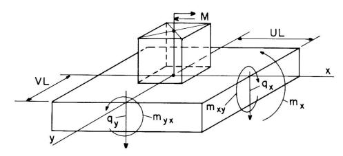
FIG. 3 SHEARS AND MOMENTS AROUND COLUMN
