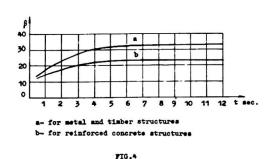
efficient is determined by means of interpolationproportional to the quantity of the potential energy stored during the oscillations of the steel and reinforced concrete parts of the structure (Fig.4ab).
