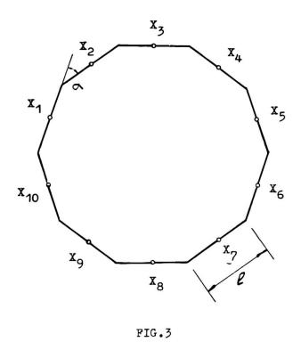
The hinges allow free rotation around the axis of the rod, that is they exclude the torsion moments but do not allow any shear or rotation around the axis perpendicular to the axis of the rod. In other words the hinge would allow the bending moments and the shearing stresses to appear. Under this assumption the design is reduced to solution of a system of fivemember equations.
