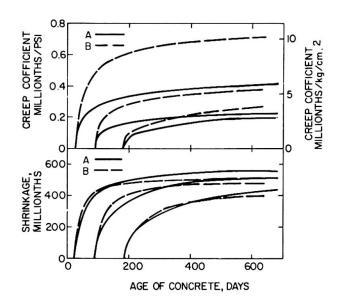
Fig. 4 - Creep and Shrinkage of Concrete
