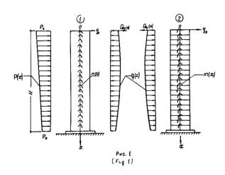
Fig. I illustrates the design scheme corresponding to the three-dimensional behaviour of structures described above with a single foundation slab under the building.
