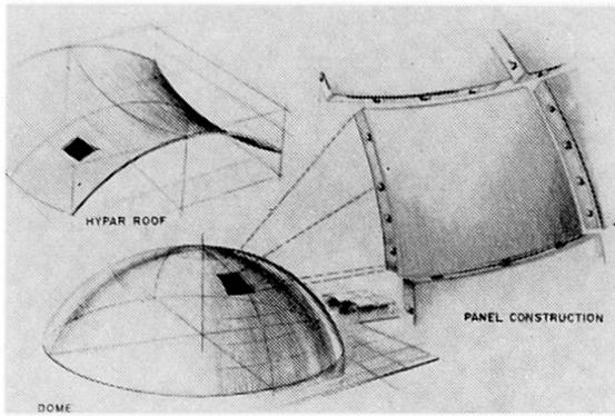
Fig. 24. Prefabricated Panels for Domes and Hypar Roofs
