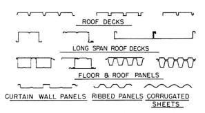
Fig. 4. Decks, Panels and Corrugated Sheets
