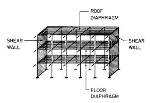
Fig. 6. Wall and Floor Diaphragms
