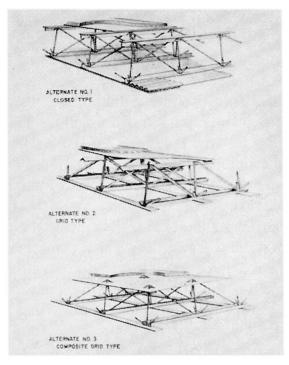
Fig. 23. Space Frame Long Span Floor Systems
