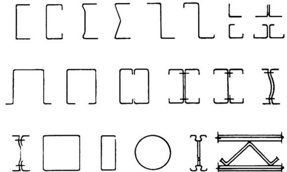
Fig. 2. Individual Cold-Formed Structural Sections
