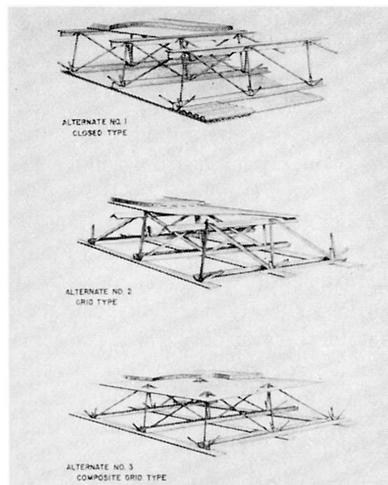
Fig. 23. Space Frame Long Span Floor Systems
