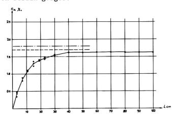
Fig. 1. Strain-increase from bar end in pretensioned bar.
