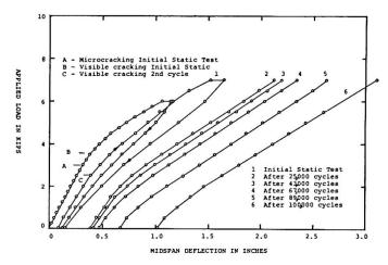
Fig. 5. Load-Deflection Characteristics After Repeated Loading, B8
