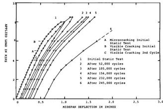
Fig. 6. Load-Deflection Characteristics After Repeated Loading, Al
