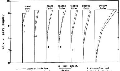
Fig. 8. Maximum Crack Width in Beam Al After Repeated Loads
