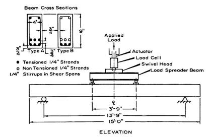
Fig. 3. Cross Sections and Loading Arrangement for Test Beams
