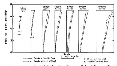
Fig. 7. Maximum Crack Width in Beam B8 After Repeated Loads
