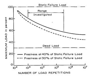
Fig. 2. Possible L-N Curves for Prestressed Concrete Beams
