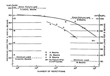
Fig. 4. Fatigue Test Results
