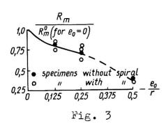
Decreasing of carrying capacity depending on the relative eccentricity of pressure load
