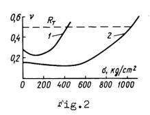
Relation between coefficient of lateral deformation (v) and stresses (6) for ordinary (1) and spiral reinforced concrete(2).
