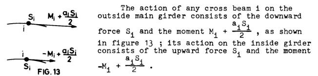
The actual deflection  $w_i$  and rotation  $\psi_i$  of the outside main girder at its junction with cross beam i under the influence of the given loading acting on the complete structural system are given by
