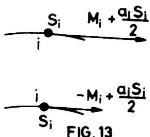
The action of any cross beam  $i$  on the outside main girder consists of the downward force  $S_i$  and the moment  $M_i + \frac{a_i S_i}{2}$ , as shown in figure 13; its action on the inside girder consists of the upward force  $S_i$  and the moment  $-M_i + \frac{a_i S_i}{2}$ .
