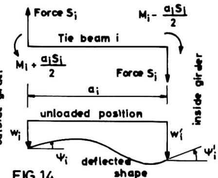
FIG.14 (I<sub>i</sub> : moment of inertia of the tie beam i).
