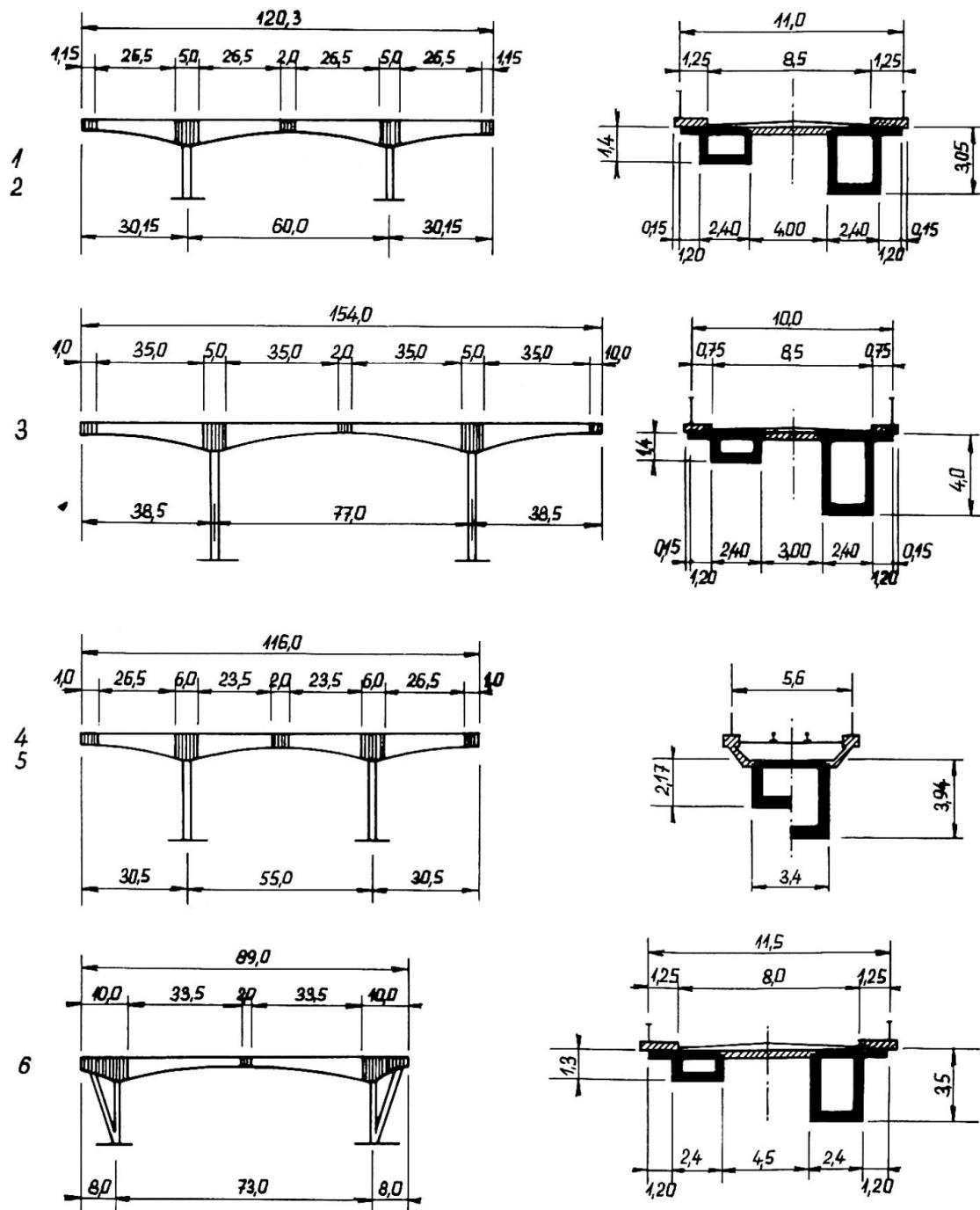
Fig. 1. Sketches of various types of the first bridges which have been erected by the new method.
