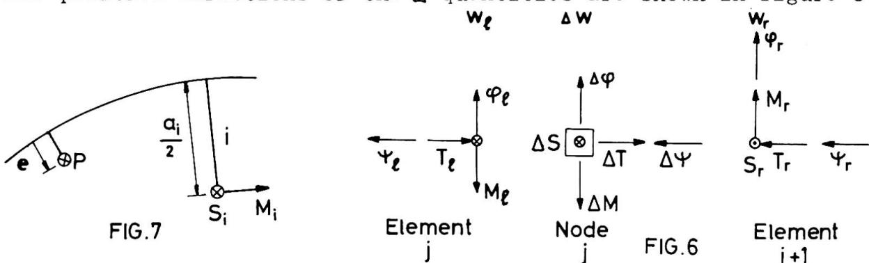
If the load consists of a downward force  $P$  acting with the eccentricity  $e$  (positive toward the center of curvature) with respect to the center line (fig. 7) :  $\Delta S = P$  and  $\Delta T = Pe$ . At the junction of the girder with the cross beam  $i$  :  $\Delta S = S_i$  and
