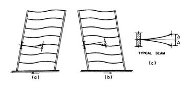
BEHAVIOR OF A FRAME IN AN EARTHQUAKE
