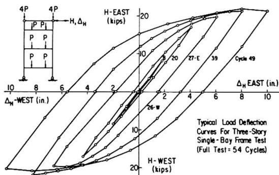
Fig. 7 Selected Load-Deflection Curves for Frame B
