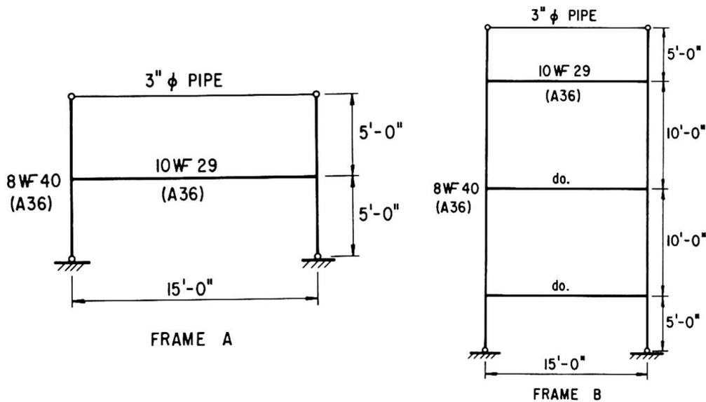
Fig. 2 Geometry and Member Sizes for Test Frames
