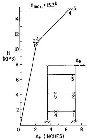
Fig. 4b Load Deflection Curve for Frame B
