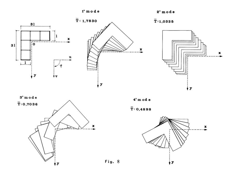
The foregoing procedure has been applied to a steel building with L plan and eight horizontal structures and with two orders of mutually orthogonal frames.
