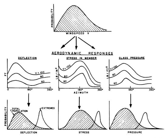
FIG. 5 DETERMINATION OF PROBABILITY DISTRIBUTIONS OF STRUCTURAL RESPONSE
