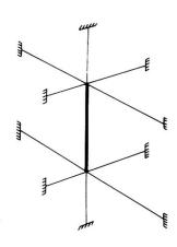
The design criterion adopted is that of attainment of yield stress at the extreme fibres in single curvature bending under factored load.
