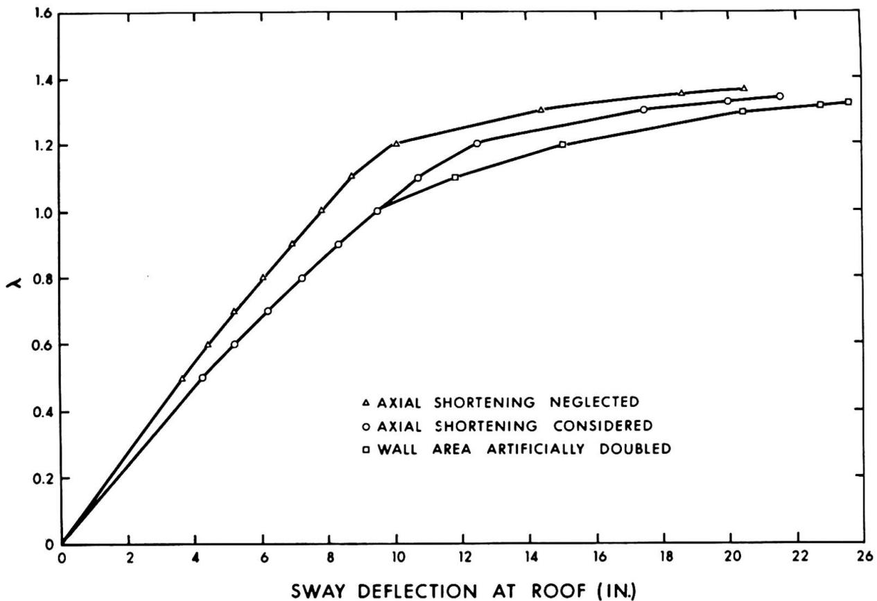
Figure 4. EFFECTS OF AXIAL SHORTENING IN FRAME H1
