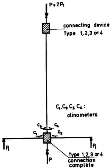
a column section supports two connections; the one at the bottom is complete, with main and secondary beam; the one at the top has only the connecting device and the beams are omitted.
