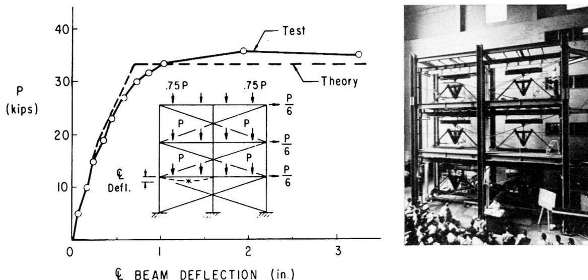
Fig. 2 Results of Braced Frame Test
