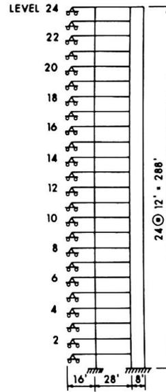
FIG. 7. LUMPED STRUCTURE
