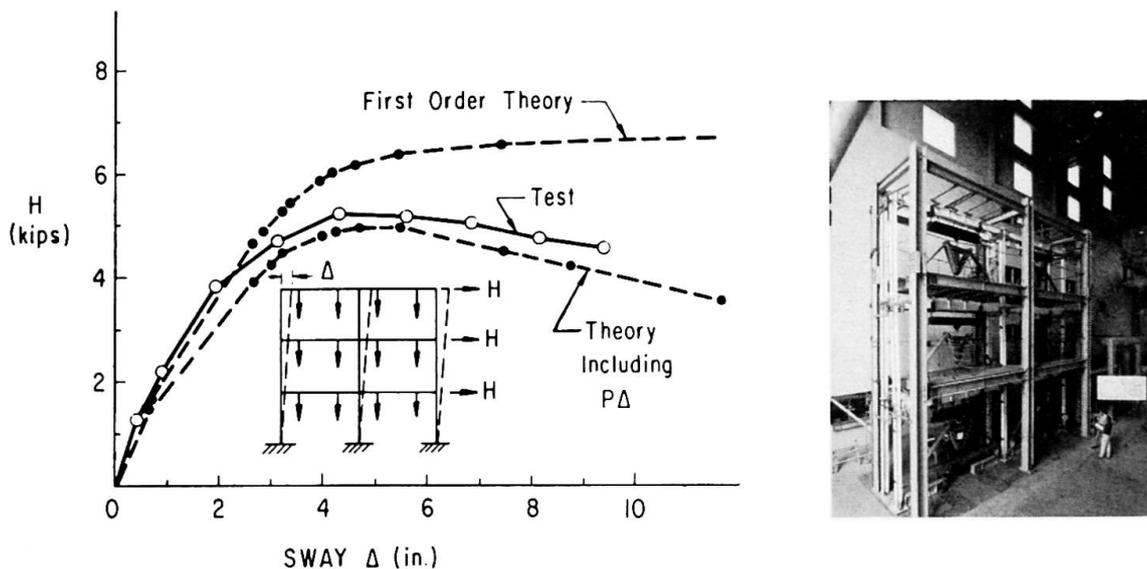
Fig. 4 Results of Unbraced Frame Tests
