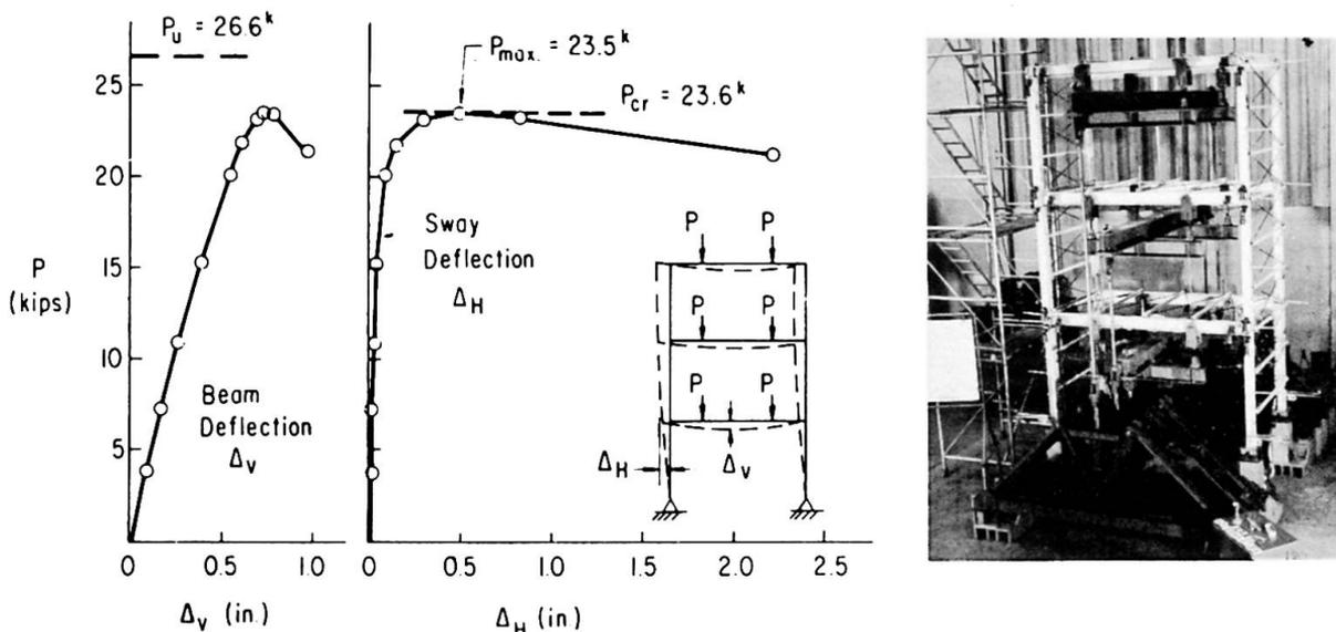
Fig. 3 Results of Frame Buckling Test
