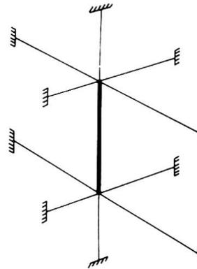
FIG 2 THE LIMITED FRAME FOR COLUMN DESIGN
