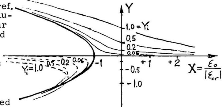
Fig. 2 Plate deflection Y versus applied edge strain X, ref [3].
