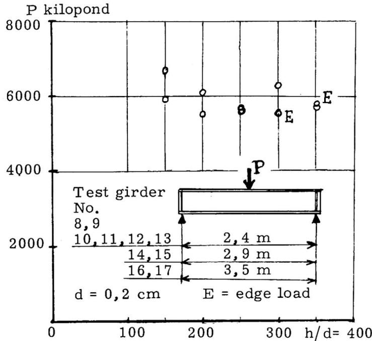
Fig. 4 Crippling loads for different web ratios.
