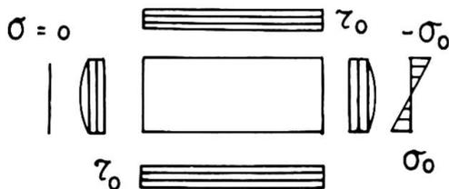
Fig. 4 Stress for Buckling Analysis
