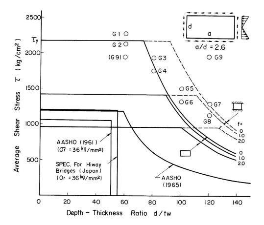
Fig. 5 Test Results and Buckling Curves
