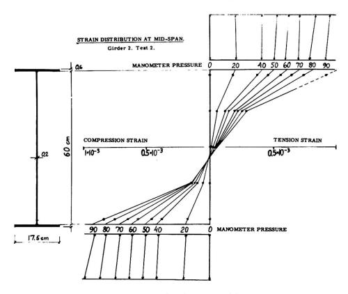
Fig. 3 Strain distribution at mid-span.
