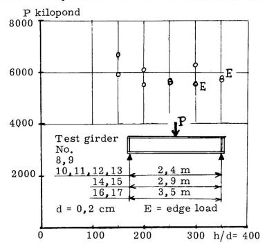
Fig. 4 Crippling loads for different web ratios.
