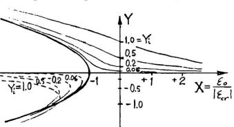
Fig. 2 Plate deflection Y versus applied edge strain X, ref [3].
