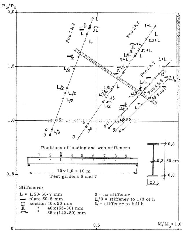
Fig. 5 Failure Loads  $P_{\rm c}/P_{\rm O}$  as function of  $\rm M/M_{\rm O}$  for different type of stiffeners.
