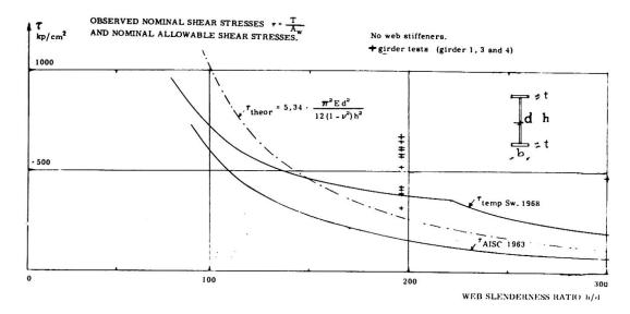
Fig. 6 Comparasion between theoretical, allowed and measured shear stresses.
