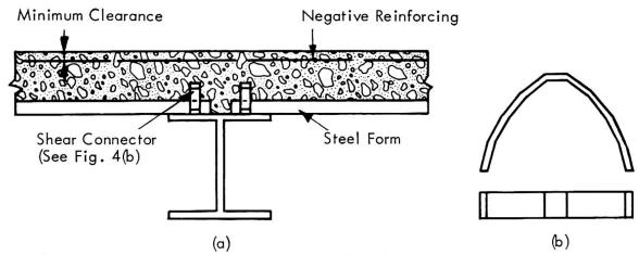
Fig. 4. Typical composite section beam detail.
