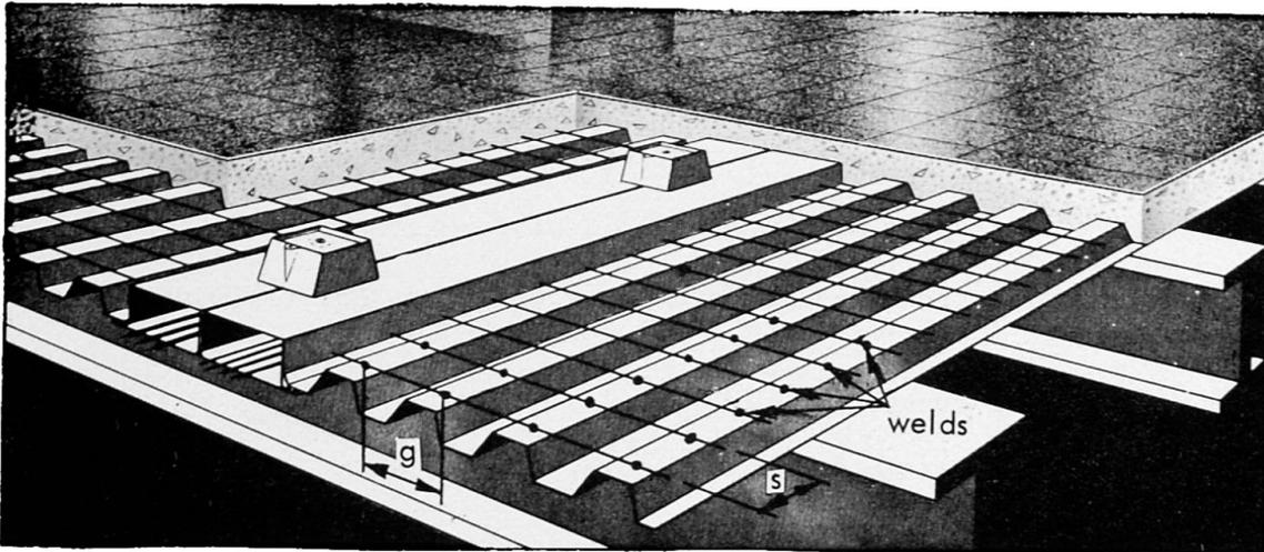
Fig. 1. Example of form which utilizes transverse wires (Category I).
