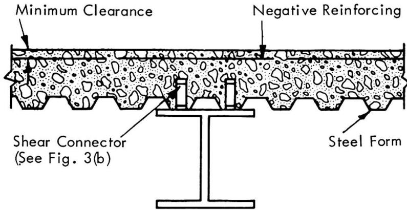
Fig. 5. Typical composite section girder detail.
