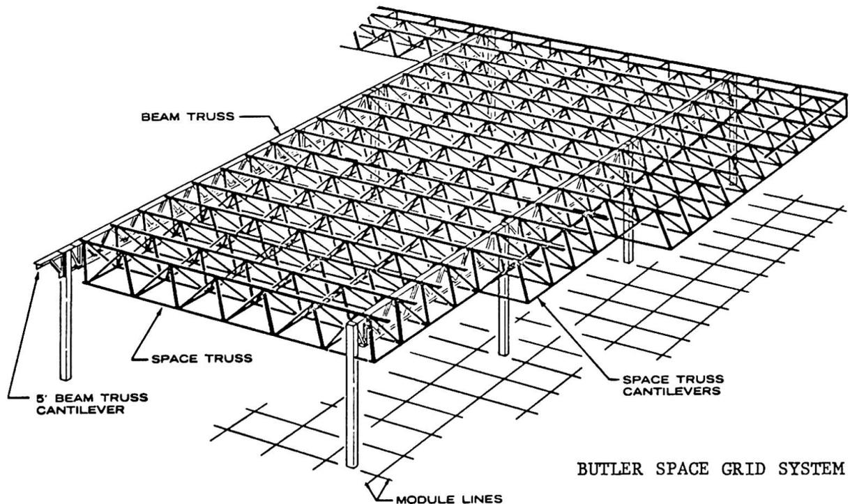
The roof covering is normally provided with an 1-1/2 inch deep light gage cold rolled steel deck which in combination with the Space Truss system acts as a diaphragm for resisting horizontal forces due to wind or earthquake.
