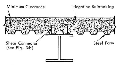
Fig. 5. Typical composite section girder detail.
