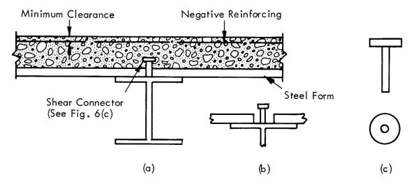
Fig. 6. Typical composite section beam detail.
