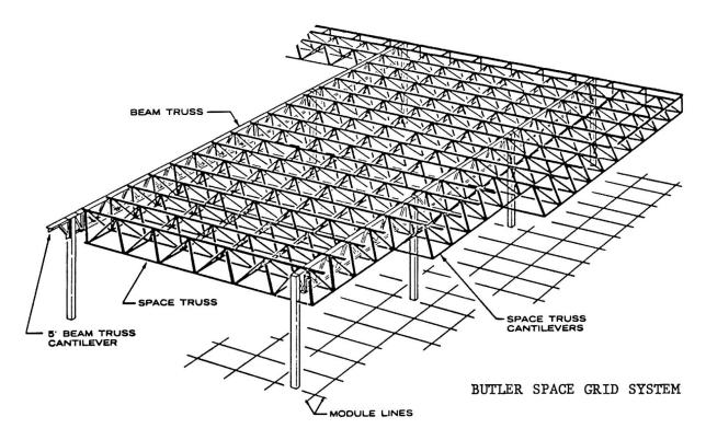
The roof covering is normally provided with an 1-1/2 inch deep light gage cold rolled steel deck which in combination with the Space Truss system acts as a diaphragm for resisting horizontal forces due to wind or earthquake.
