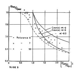
constant of proportionality and ← = 0 is of course the results for a perfect plate. The experimental results in this figure are for square tubes, both aluminium and steel. Slide (3) shows corresponding results for steel and aluminium plates. The greater scatter is attributed to defective edge boundaries.
