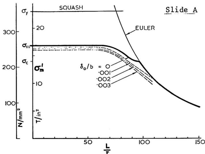
The interesting thing on all the curves is the long flat portion, showing that the full section strength can be developed up to a considerable member length. In slide B, which refers to the same section, these results are compared with two current design philosophies, curve 3 being Grave Smith's theoretical one for a member having a small initial waviness. In heavy steel design it is common to use a simple "effective width" procedure, in which one
