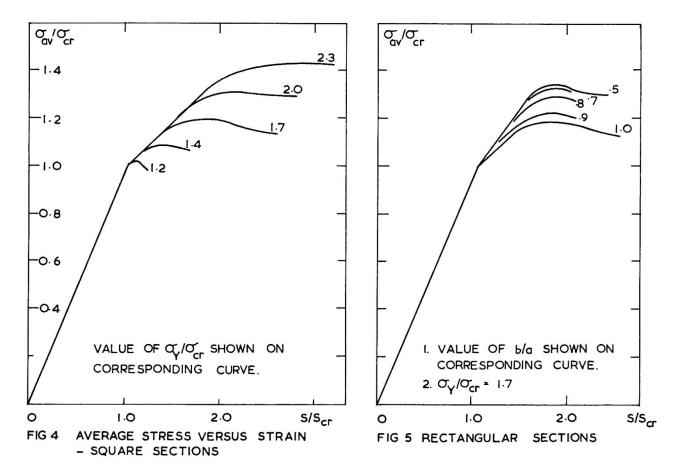
An interesting feature of the results is that the corners of the columns go completely plastic in a predominantly compressive mode at about the same time as the ultimate load is attained, which lends support to the 'equivalent width' design approximation discussed by Professor Winter. The theoretical results for the square column agree well with the results of some simply supported plate tests recently reported by Dwight and Ractliffe<sup>9</sup>.
