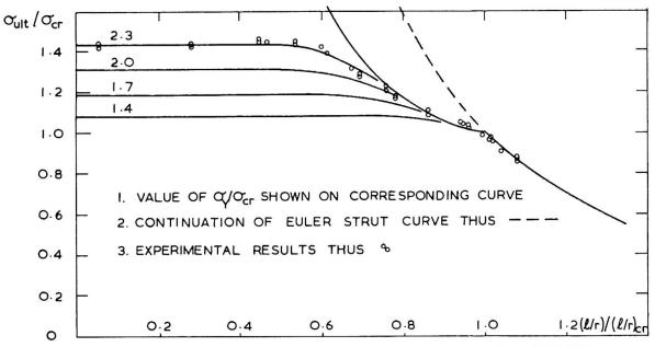
FIG. 7 ULTIMATE STRESSES OF SQUARE THIN WALLED COLUMNS
