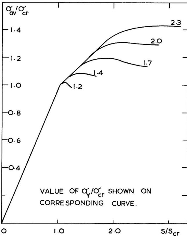
FIG 4 AVERAGE STRESS VERSUS STRAIN - SQUARE SECTIONS
