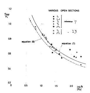
Fig. 8 Results of tests on various open sections of aluminium-alloy materials.
