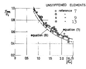
Fig.5 Results of tests on unstiffened plate elements of aluminiumalloy materials.
