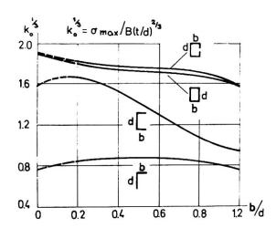
Fig.9 Values of the constant & for a number of shapes of cross-section of uniform thickness.
