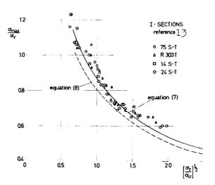
The results of tests on channel sections by Heimerl (ref.9) and Gerard (ref.13) are shown in Fig.6, on I-sections by Gerard (ref.13) in Fig.7 and on a variety of open sections reported by Needham (ref.7) and Gerard (ref.13) are shown in Fig.8. Again, the test results in the case of sections are described reasonably accurately by equation (7).
