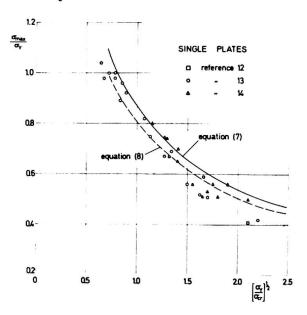
Fig. 4 Results of tests on compressed square tubes of aluminium-alloy materials.
