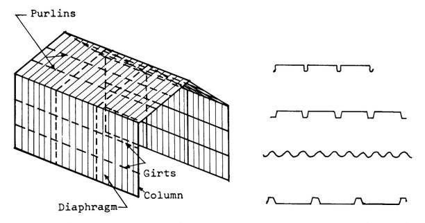
Fig. 1 A Steel Framed Building Fig. 2 Panel Configurations
