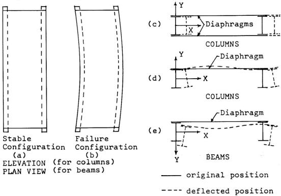
Fig. 3 Diaphragm-Braced Columns or Beams
