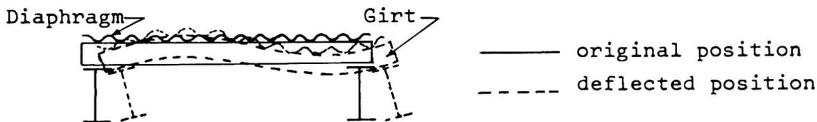
Fig. 4 Columns with Diaphragm-Girt Bracing
