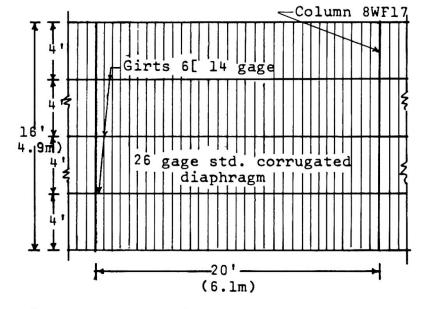
Fig. 11 Column-Girt-Diaphragm Assembly of a Typical Steel Building
