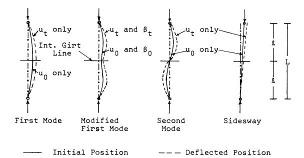
Fig. 5 Buckling Pattern of an Imperfect Column with One Intermediate Girt
