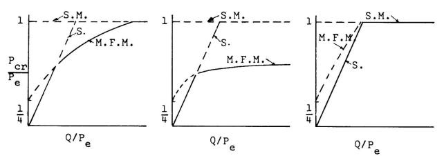
Legend: M.F.M. - Modified First Mode, S.M. - Second Mode, S. - Sidesway, as shown in Fig. 5;  $P_e = \frac{\pi^2 EI_V}{\ell^2}$
