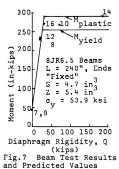
buckling loads with test failure loads for 8JR6.5 assemblies is shown in Fig. 7. The moments sustained by the diaphragm-braced beams were always more than 80% of predicted buckling values for ideal members, and as high as six times the buckling moments of corresponding unbraced beams.
