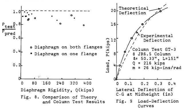
Columns with Diaphragm-Girt Bracing - Tests were made on three assemblies of axially-loaded pairs of 8JR6.5 I-section columns braced by two intermediate girts and a 26 gage standard corrugated steel diaphragm. Columns were spaced 6' (1.8 m) apart and were
