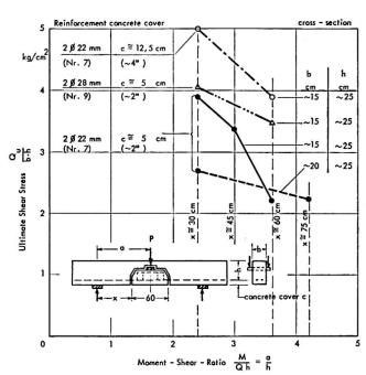
thickness of the concrete cover, the percentage of the longitudinal reinforcement and last but not least with decreasing shear span or M/Qh. The dowelaction follows, therefore, quite closely the tendencies of the phenomena mentioned so far, and one could be tempted, to consider it as their major cause.
