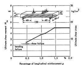
Fig. 3. Influence of the percentage of longitudinal tension reinforcement on the ultimate shear-moment of simply supported slabs.
