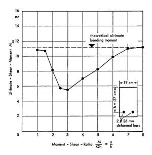
Fig. 2. Evaluation of the same test results as given in Fig. 1 (upper curve), but in terms of ultimate shear-moment.
