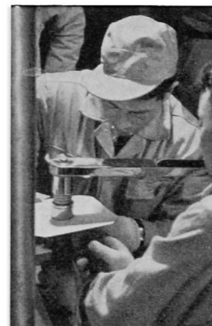
Fig. 10. Bolt tightening test by use of load cell.
