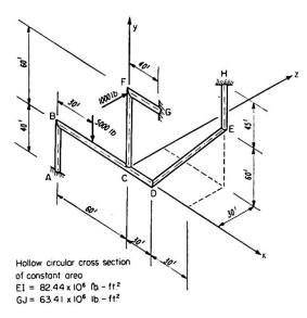
Fig. 2. Structure for numerical example.
