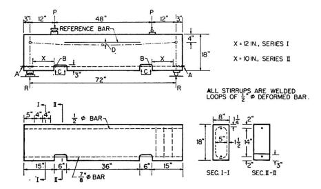
Specimens cast erect — main  $^{7}/8'' \varnothing$  steel bar in bottom. Specimens cast inverted — main  $^{7}/8'' \varnothing$  steel bar in top.
