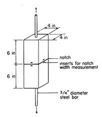
Fig. 4. Corrosion Specimen Details.
