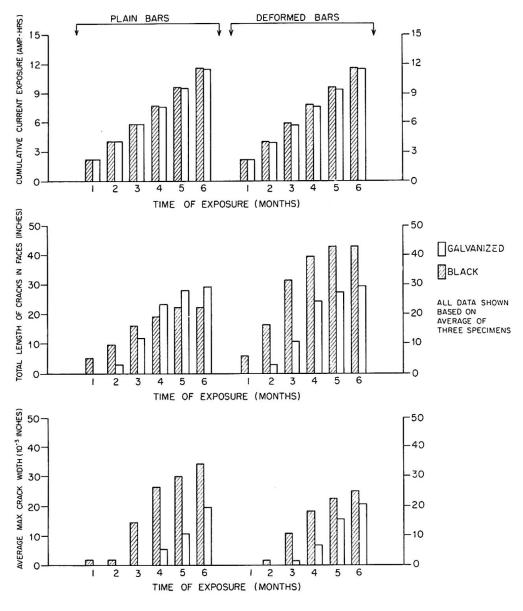
Fig. 6. Corrosion Performance Under Sustained Direct Current.
