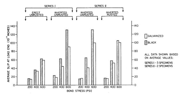
Fig. 3. Bond Performance of Deformed Bars.
