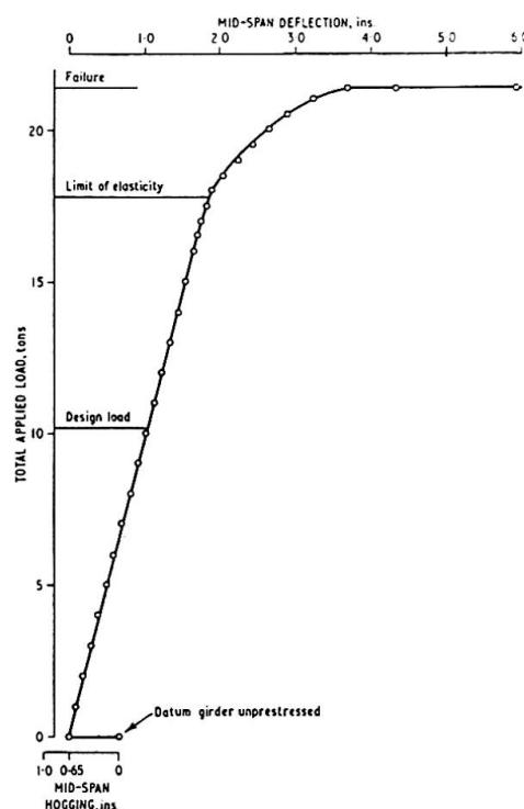
Fig. 7. Load/Deflection relationship of model delta girder.
