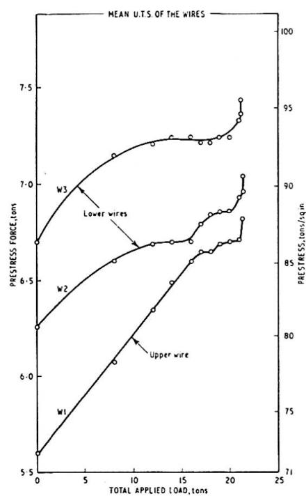
Fig. 8. Prestressing bar forces of model delta girder.
