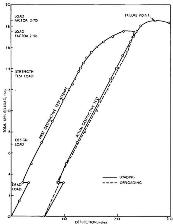
Fig. 4. Load/Deflection relationship of model lattice girder.
