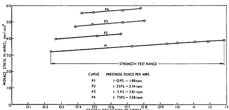
Fig. 5. Prestressing bar forces of model lattice girder.
